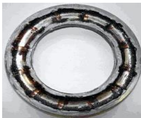
Figure I.6: corrosion de roulement
