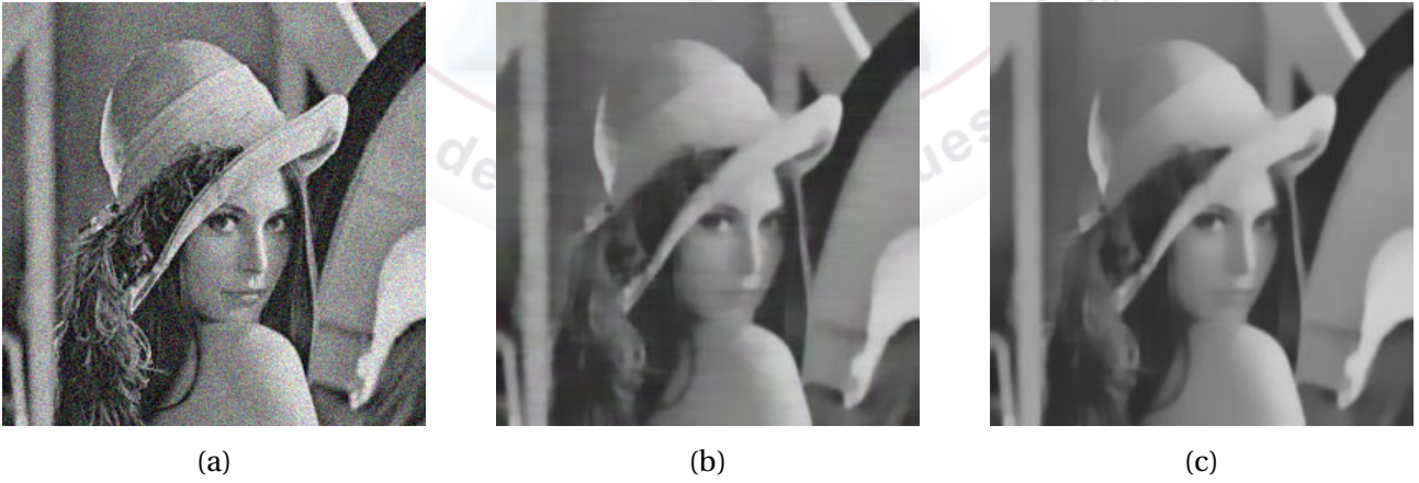
Figure 2.4: (a) Original image. (b) Denoised image by Perona-Malik model. (c) Denoised image by regularized Perona-Malik model.
