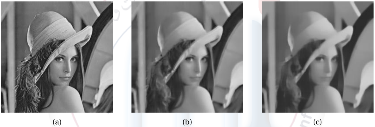
Figure 3.2: Comparison of different filtering models after 20 iterations. From left to right: original images, smoothed original image by the fractional Perona-Malik model for \alpha = 0.1 and smoothed original image by Catté and al. model, respectively.
