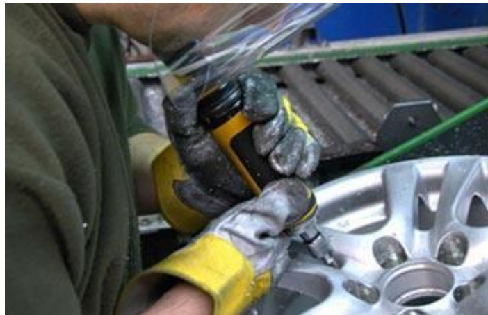
Figure III.23. Ebavurage et finition de la jante [55].
