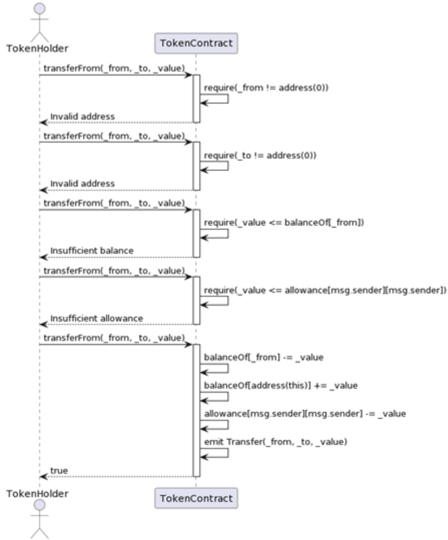
Figure 28: Sequence diagram of TransferFrom
