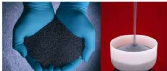
Figure II 4 Crystal Growth Efficiency with Fluidized Bed Reactor-Produced Granular Polysilicon. [14]
