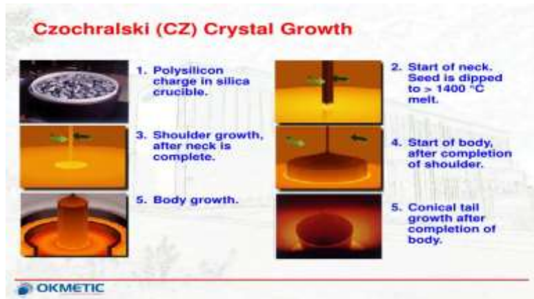
Figure II 6 The Czochralski method [15].
