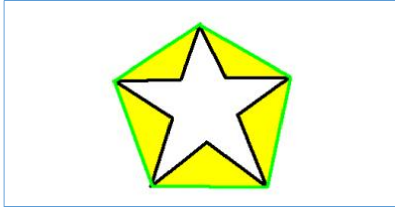
Figure 3.35 Yellow parts represent the convexity defects
