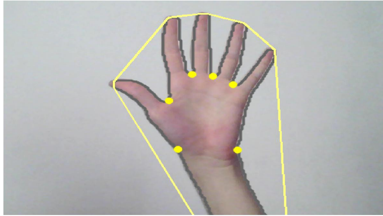
Figure 3.41 Remove depth points which have small depth
