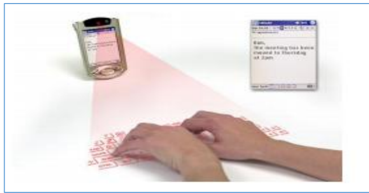
Figure 1.12 Canesta virtual keyboard
