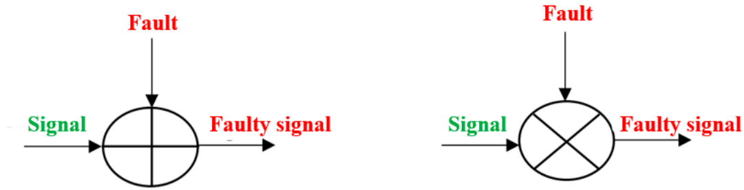
Figure 1. 4 - Classification of faults. (left) additive faults, (right) multiplicative faults
