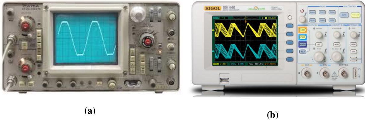
Figure 1.6. Oscilloscope: (a) analog oscilloscope and (b) digital oscilloscope.
