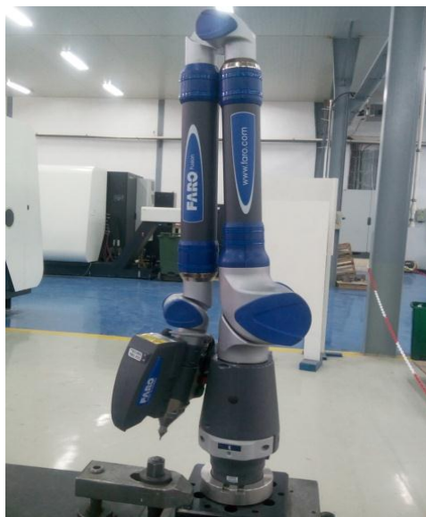
Figure III.1 : Scanner 3D de type FARO (MEI SONLGAZ M'sila).
