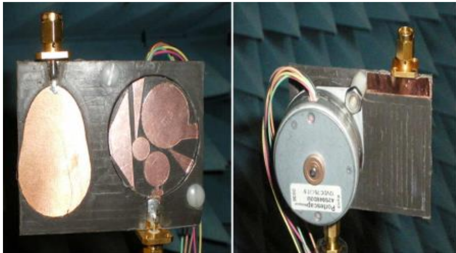
Figure II.4: Geometrical (mechanical) reconfiguration of an antenna [23].
