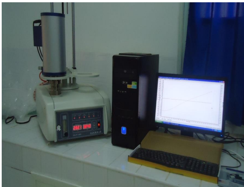
Figure II.4: Appareil TG: 70/217Thristor-Power supplylinse
