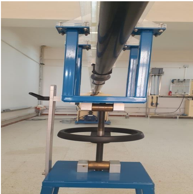
Figure I.6: dispositif de variation de pente
