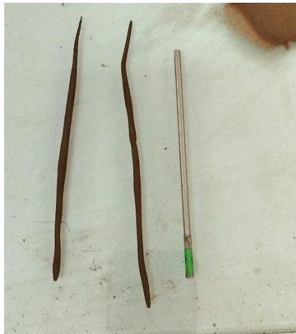
Figure 9. Plastic limit test using the rolling method
