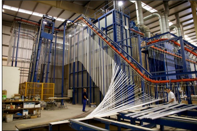
Figure III -18 : Processus Thermo Laquage
