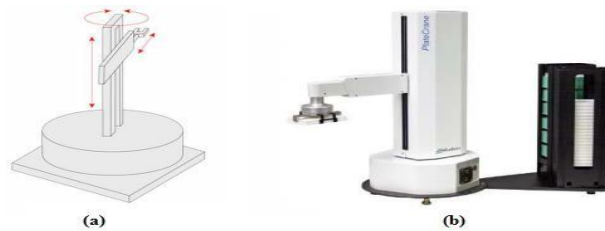
Figure.I.17 : (a) Structure cylindrique, (b) Robot cylindrique (Plate Crane) [1]
