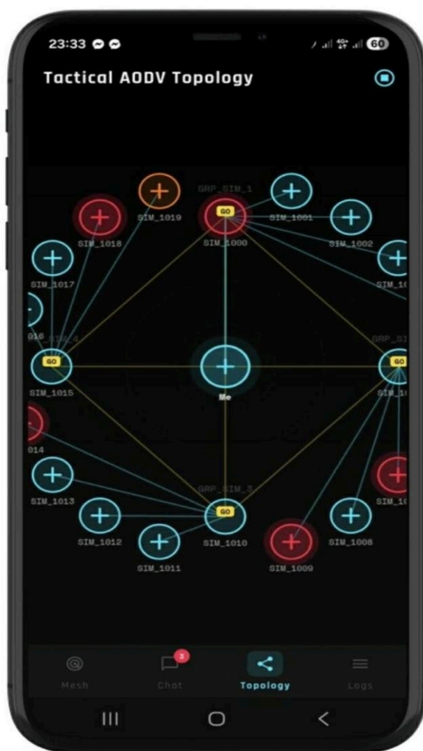
Fig. 3.13: Topology — Full 20-Node Simulation: 4 Groups (GRP_SIM_1 to GRP_SIM_4), GO Badges (Yellow), Bridge Edges (Orange), Red SOS/Victim Nodes
