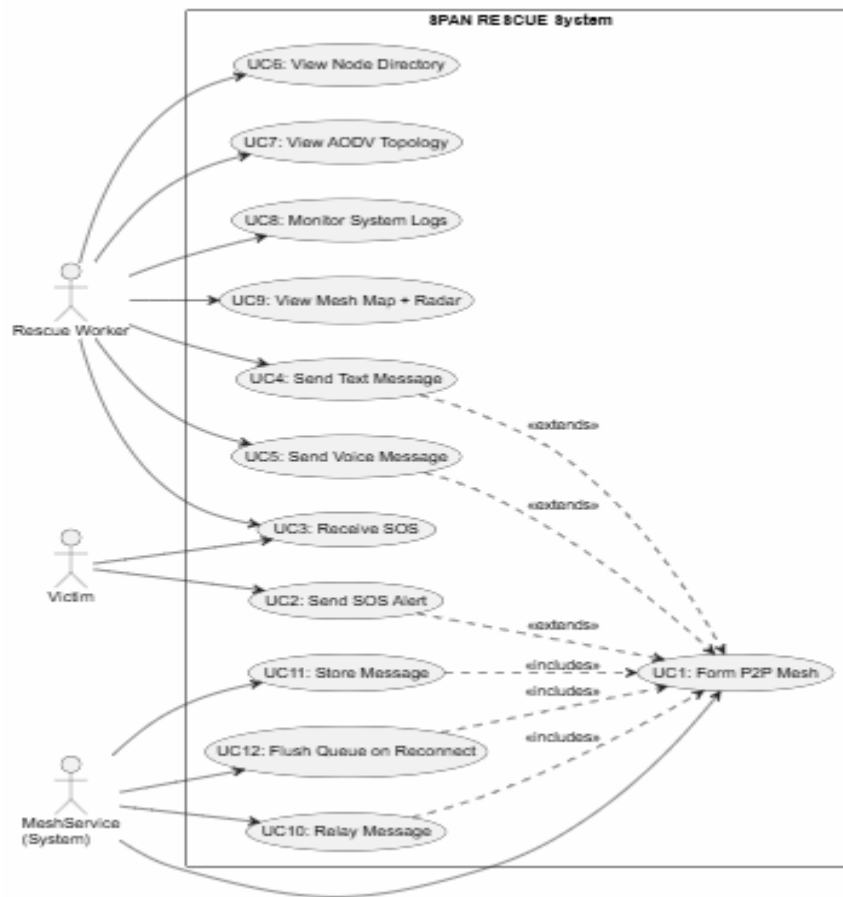
Fig. 2.11: UML Use Case Diagram — Actors, Use Cases, and Dependencies
