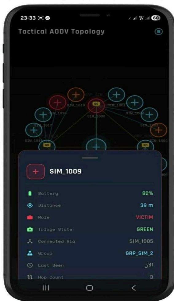
Fig. 3.14: Node Detail Panel — SIM_1009: Battery/Role/Triage/ConnectedVia/Group/HopCount
