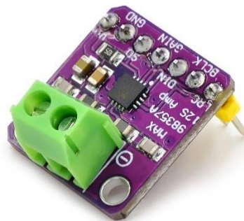
Figure 4: MAX98357 DAC Amplifier
