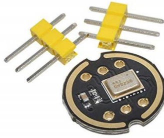
Figure 5: INMP441 MEMS I2S Microphone Module
