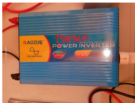
Figure III.17 Onduleur RGS - 1500 W.
