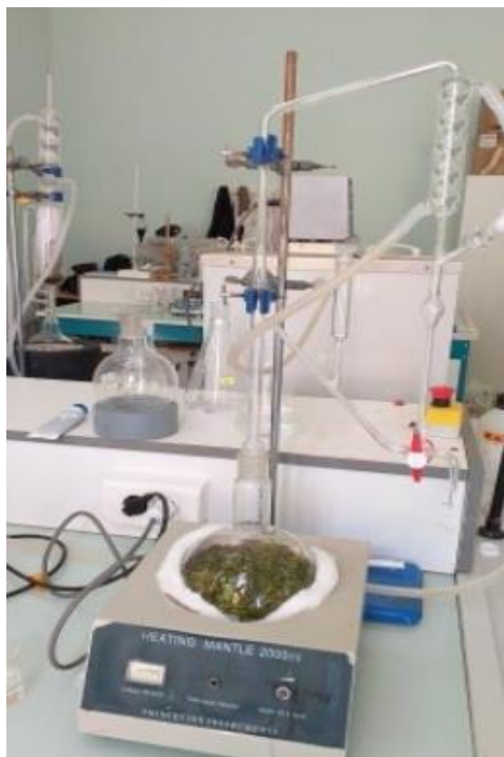
Figure II.4. The essential oils extraction of C. phelypeae by Clevenger
