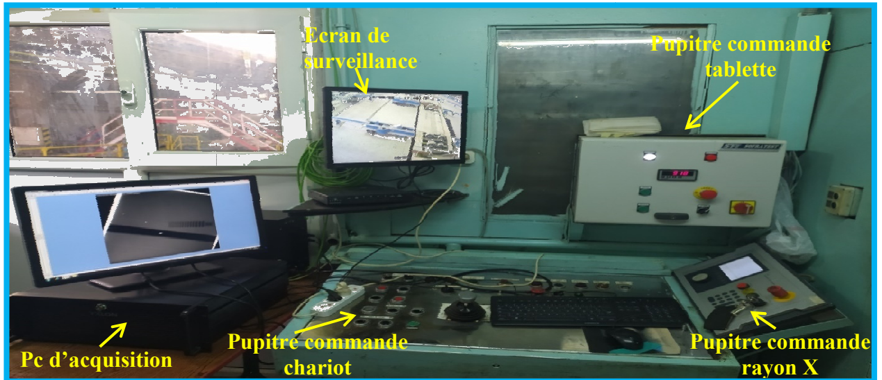
Figure IV. 7 Station d'acquisition d'image.
