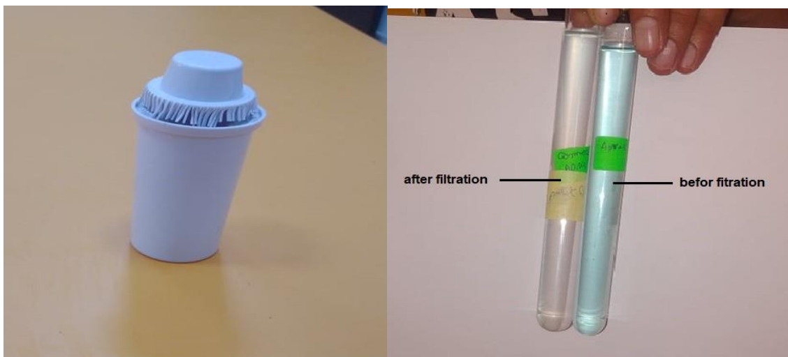
Figure IV.22 Photos showing the color change of the methylene blue solution before and after filtration (commercial Activated carbon of Filter II)
