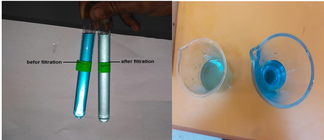
Figure IV.23 Photos showing the color change of the methylene blue solution before and after filtration (local Activated carbon)
