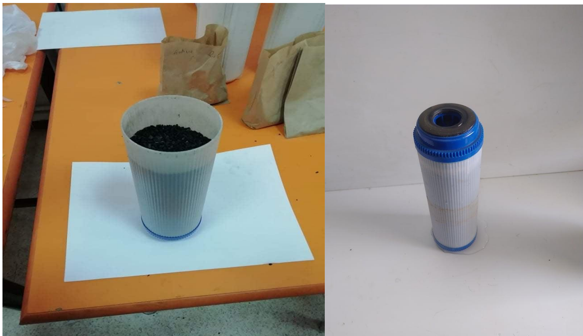
Figure IV.18 Preparation of our GAC filter using an existing packaging
