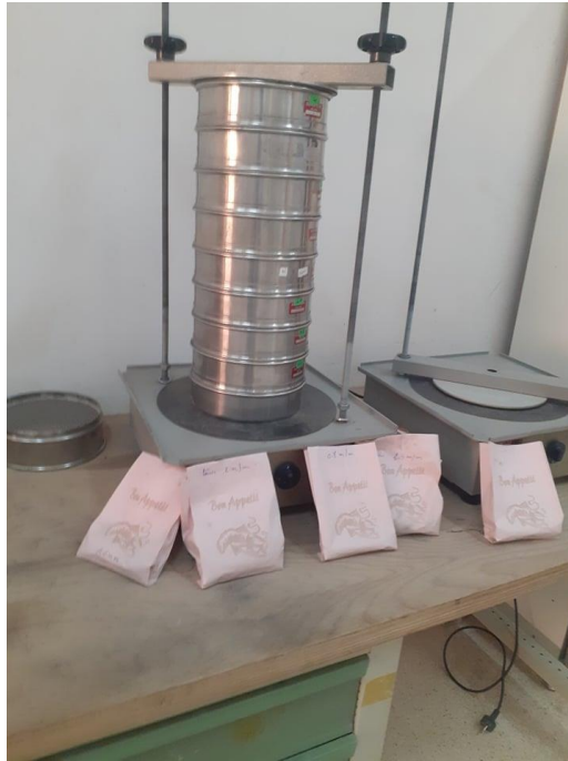
Figure IV.14 Selection of sieves to have the same grain dimensions as those of the commercial filter
