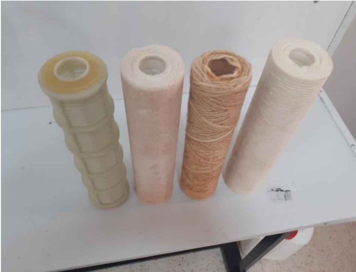
Figure II.4 Real picture of Sediment Filtration
