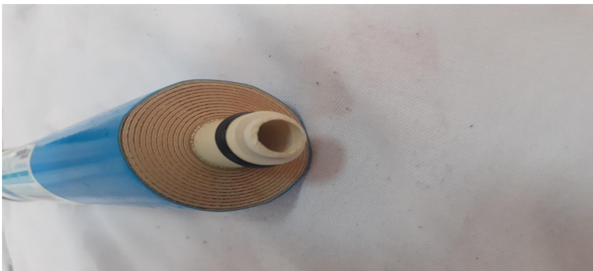
Figure II.14 Real picture of R.O. Membrane (spiral wound membrane)
