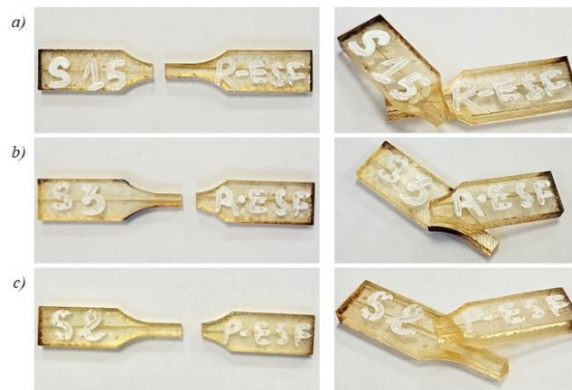
Figure IV. 15. Photographs of fracture facies of model composites: a) R ESF , b) A ESF and c) P ESF with Epoxy matrix after the tensile test
