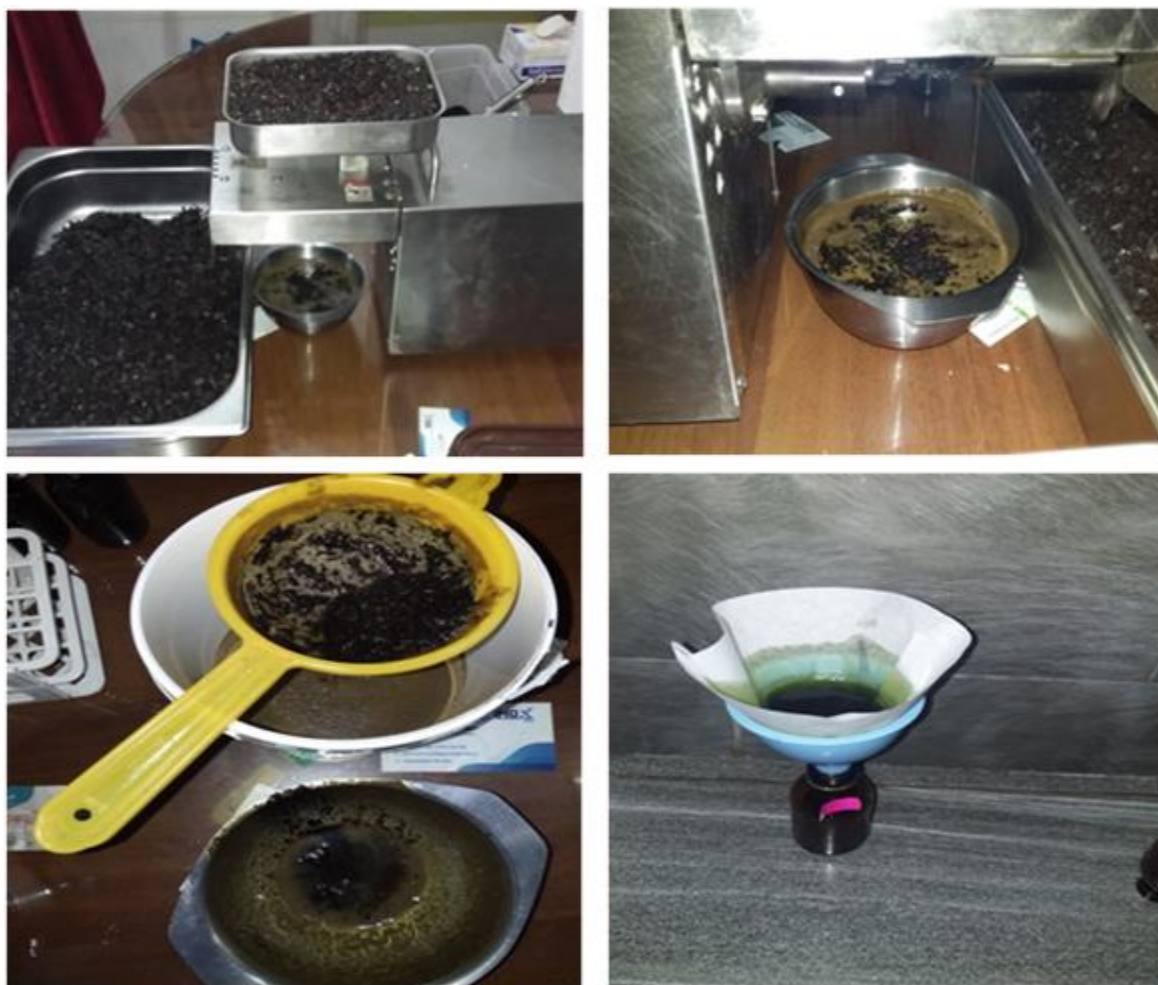
Figure 11: Operation of extraction by cold pressing.
