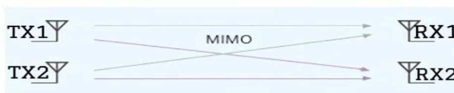
Figure 2.15: MIMO Multiple Input Multiple Output
