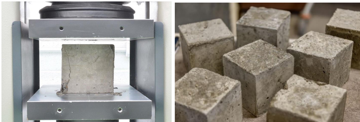
Figure 40: compression test specimens
