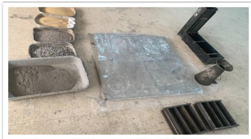
Figure 31 : Preparations of concrete specimens
