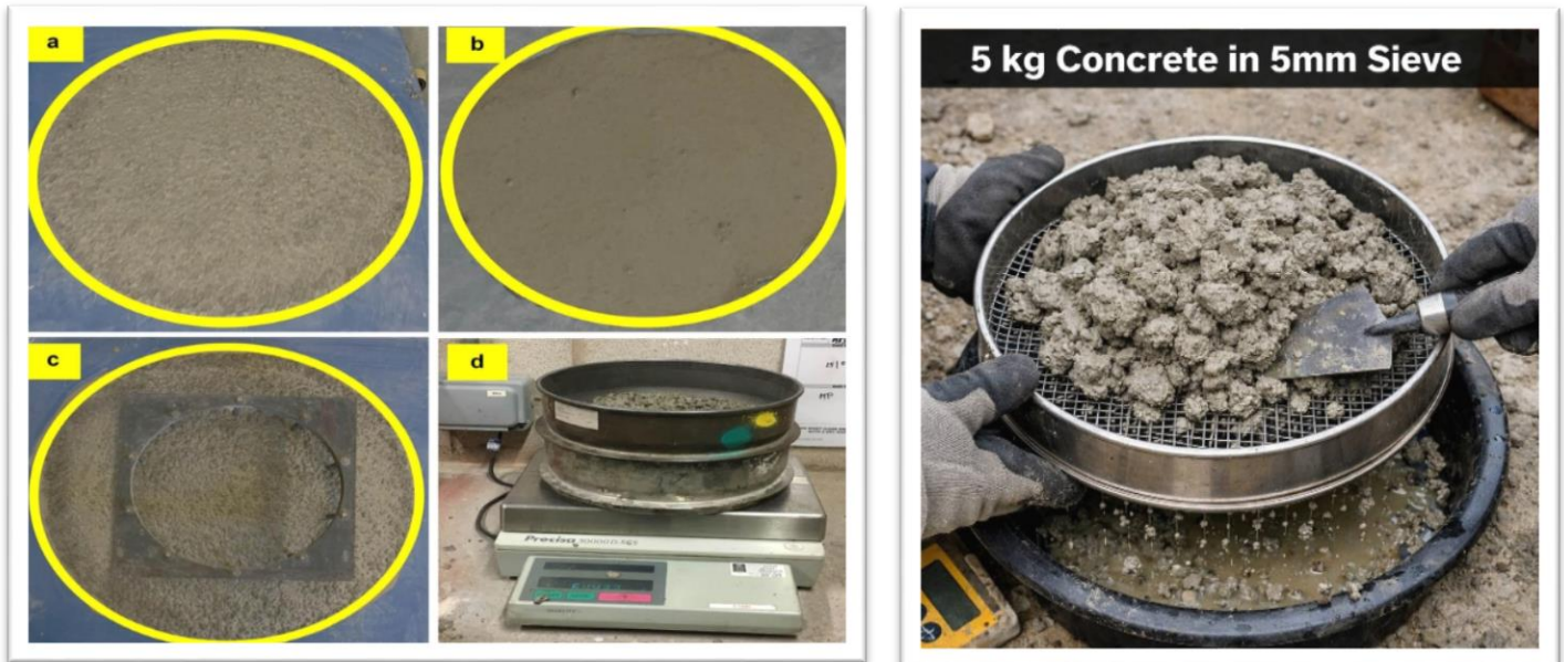
Figure 6: Representation of the sieve stability test
