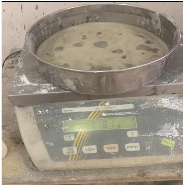
Figure 36 : Sieve stability test principle for SCC
