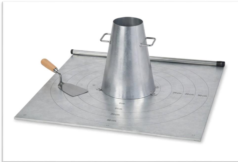
Figure 3: Slump flow test with Abrams cone.
