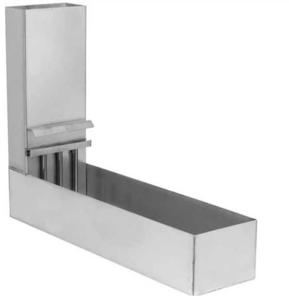
Figure 5: Schematic representation of the L-box test
