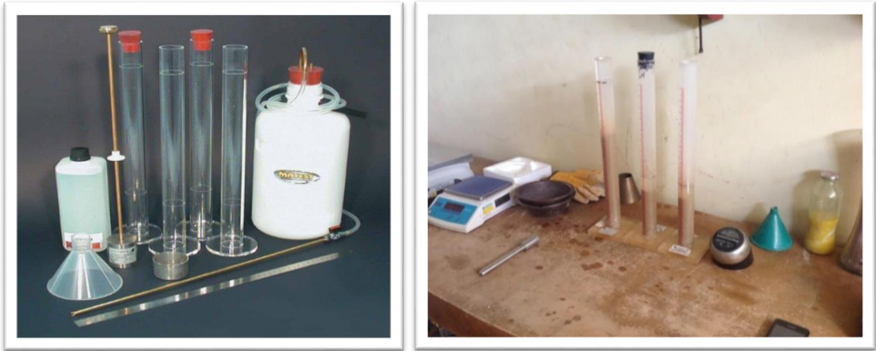
Figure 22 : Principle of the Sand Equivalent Test
