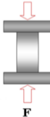
Figure .III.5. Essai de compression [12].
