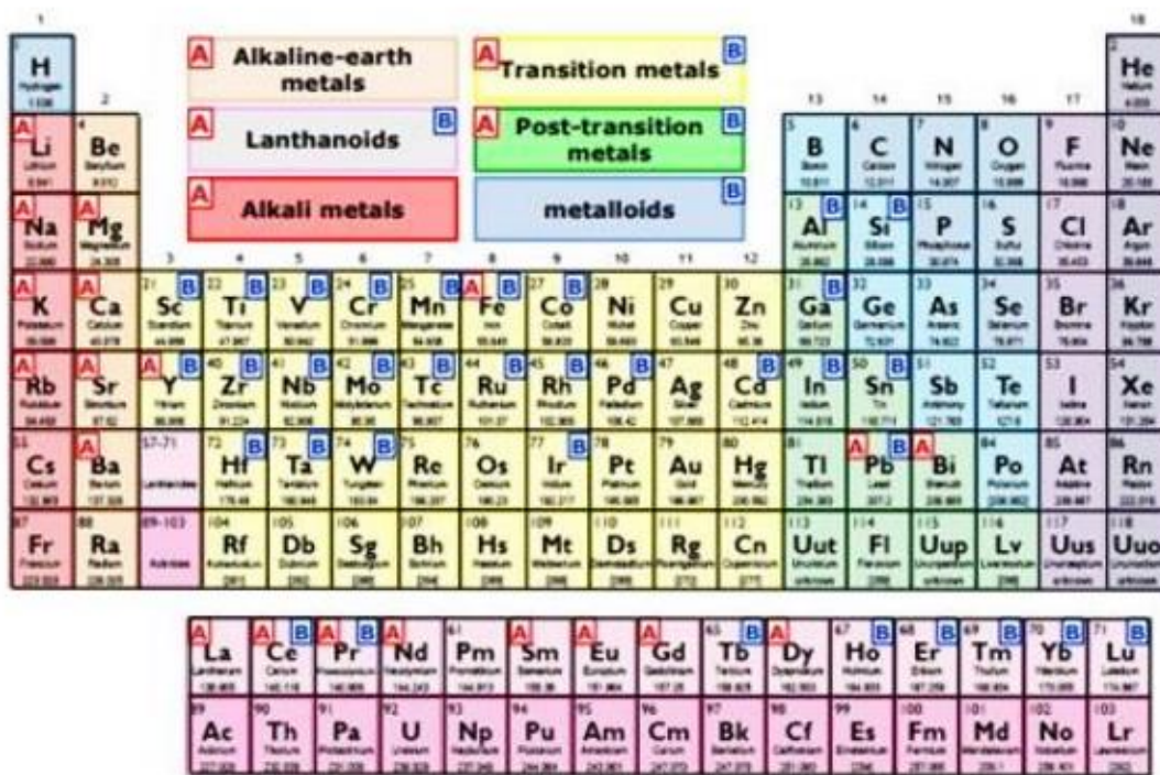
Figure 1.3. Periodic table of atoms that can be accommodated on the A and B sites of the perovskite lattice.
