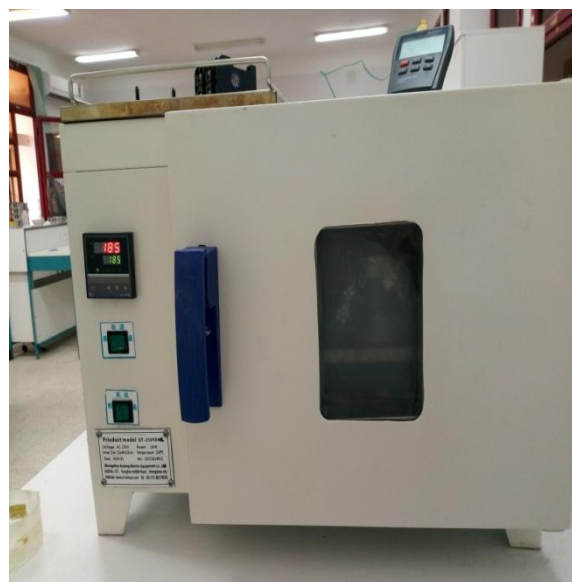
Figure III.8: Etuve de type UNB 400.
