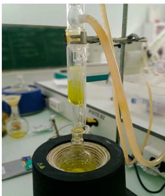
Figure 11: Montage de type Soxhlet
