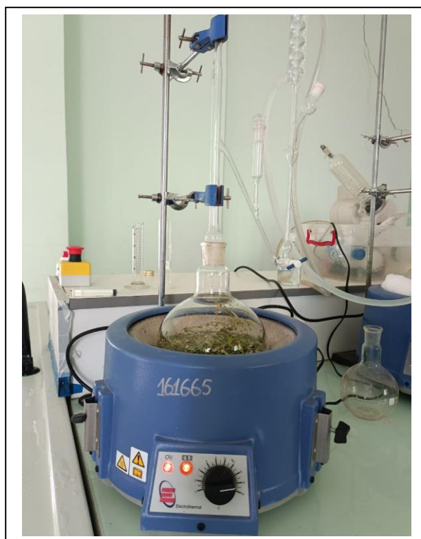
Figure 15: montage de type Clevenger
