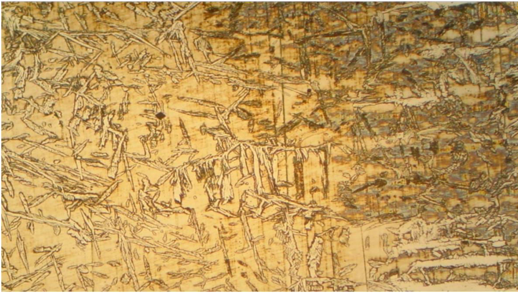
Figure IV.6 : Microstructure la ZL d'acier (2205) GX200
