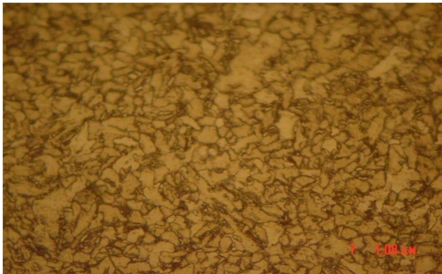
Figure IV.5: Microstructure la ZAT de A106 GX200
