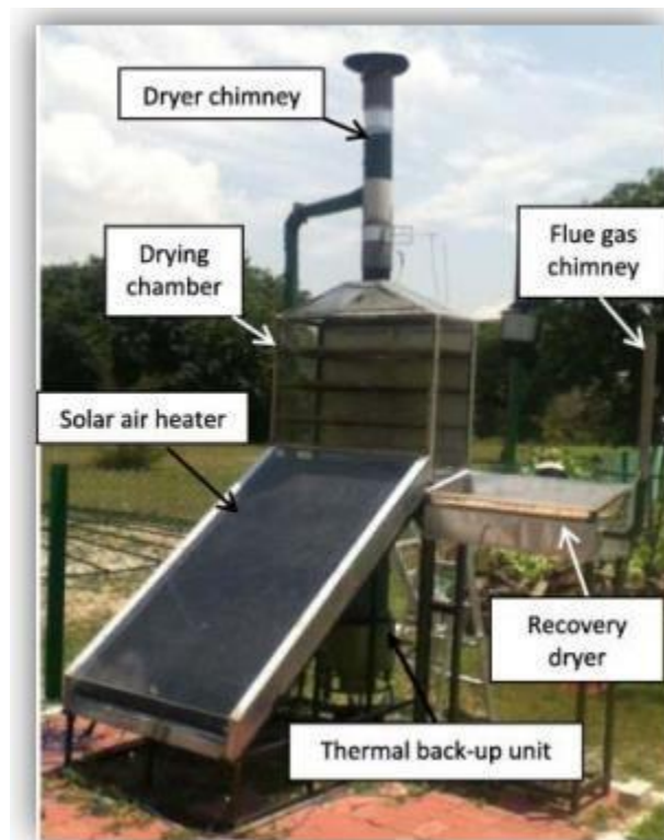
Figure II.22 Séchoir solaire hybride.
