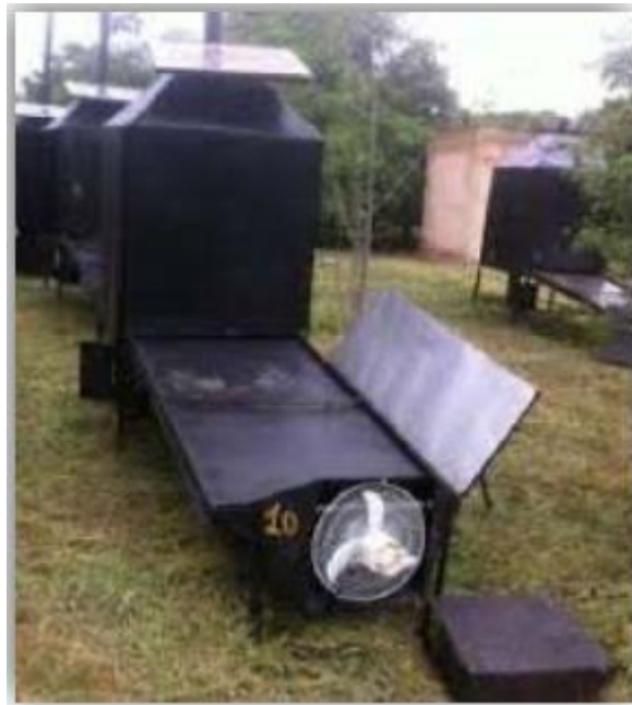
Figure II.23 Séchoir solaire hybride à convection forcée
