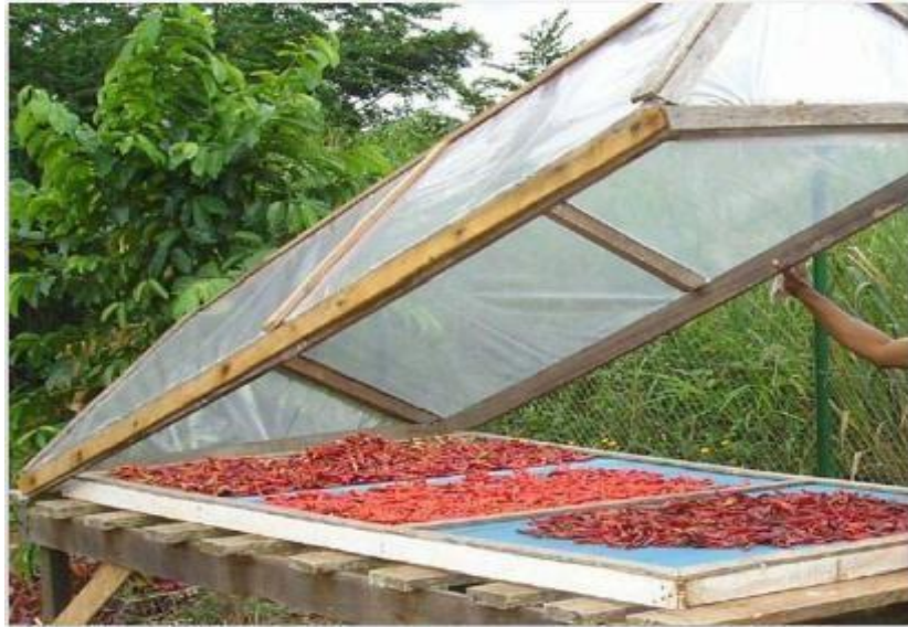
Figure II.6 Séchoir solaire "Tente".
