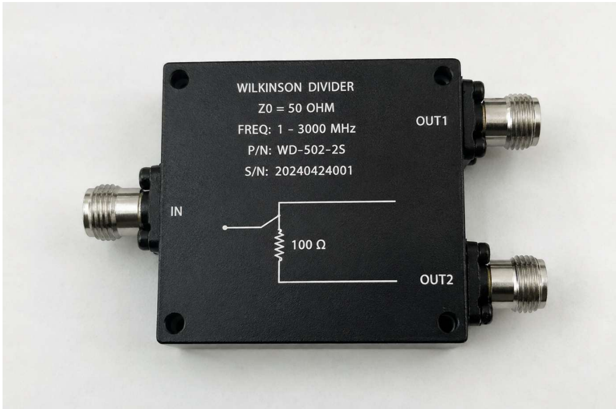
Figure 2.9 Photograph of Wilkinson Power Divider with Z_0 = 50 \Omega .
