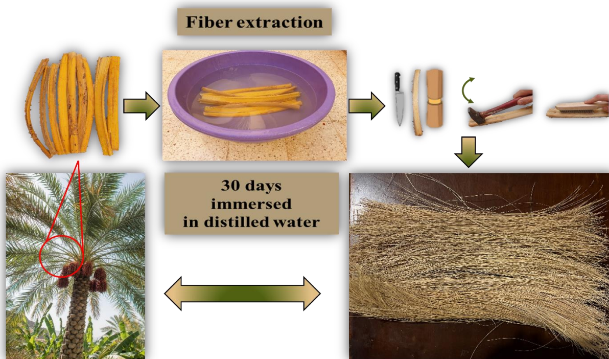
Figure II-1: The different steps for fiber extraction.
