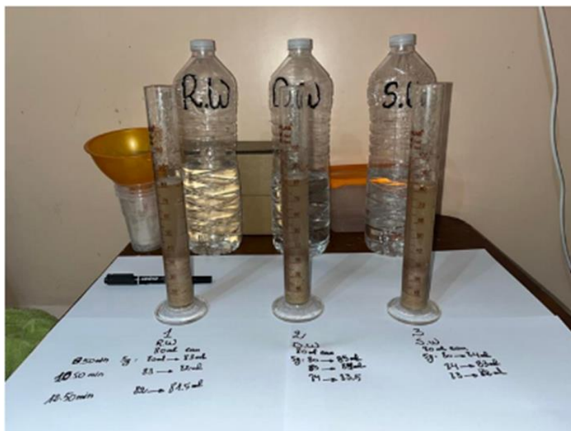
Figure II-5: Water absorption evaluation of date palm fiber (DPF).
