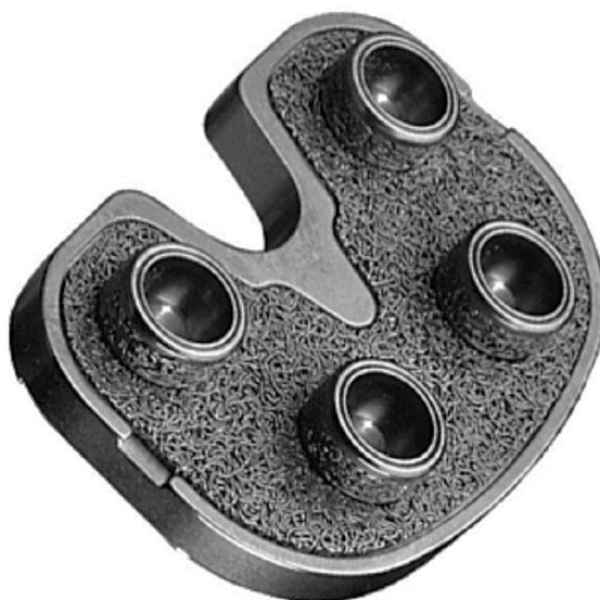
Figure I-15: NexGen porous titanium fiber-mesh (Ti) tibial metal-backing with 4 short pegs for screw fixation in the proximal tibia[96].
