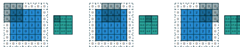
FIGURE 1.18: Convolution with zero padding and stride > 1 . Only the 1 st three subplots are shown here. Padding is of depth 1, stride is 2, and filter size is 3 \times 3 [25].
