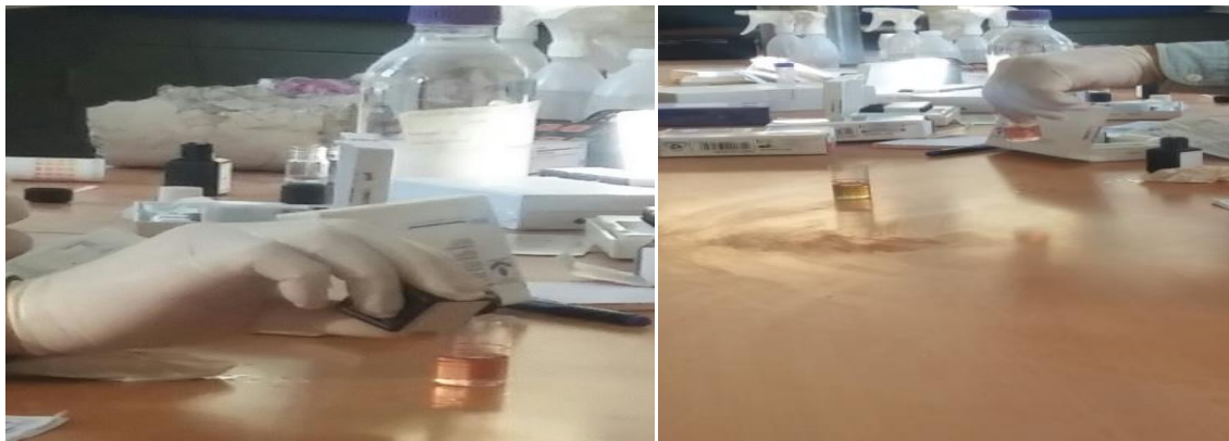
Figure III.14 essai de Test Dureté totale
