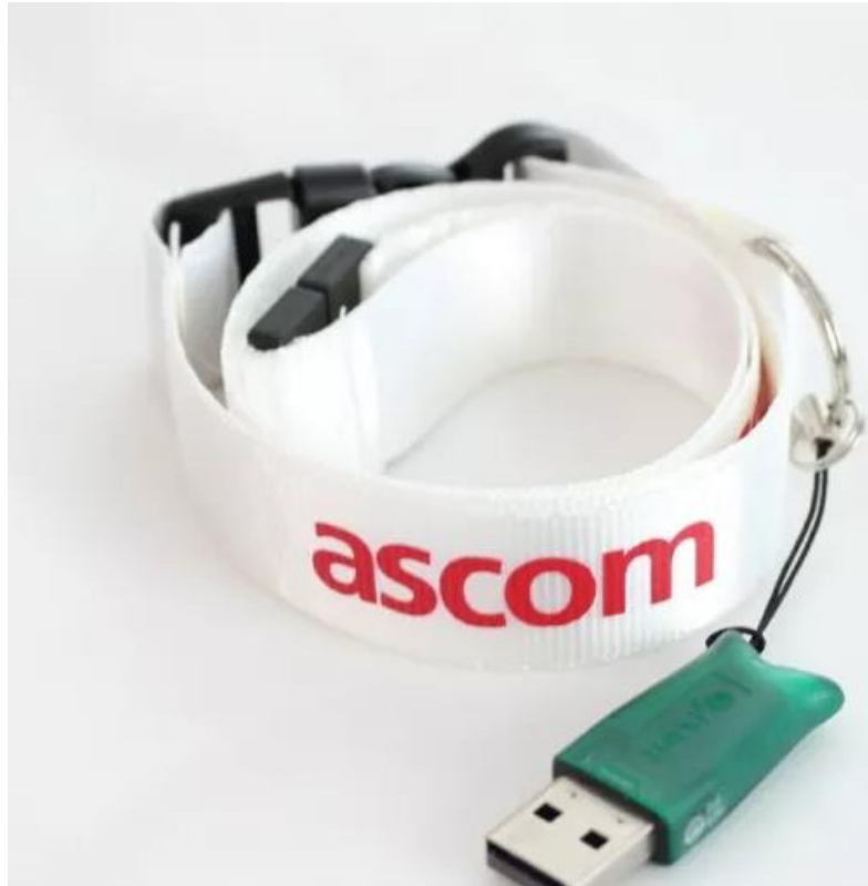
Figure IV.5 : Dongle TEMS investigation [20]
