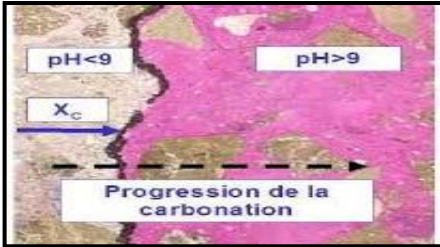
Figure II.15. Progression du front de carbonatation.
