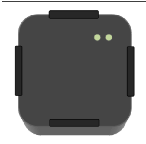
Figure 2.4: Basic design of robot with 4 collision sensors.
