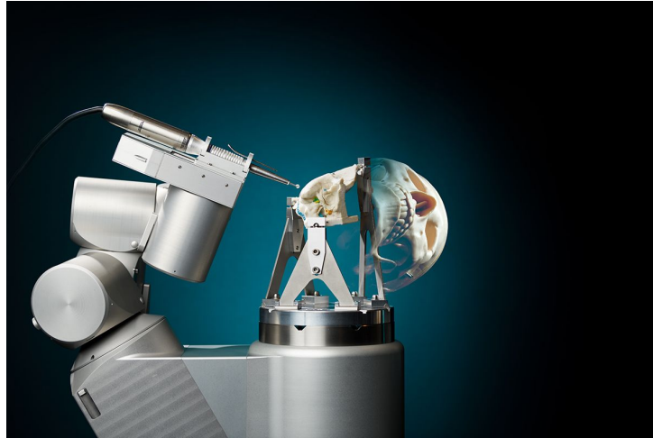
Figure 1.3: This is the skull bone surgery robot RoBoSculpt, developed by Jordan Bos of Eindhoven University of Technology. On the right there is a phantom piece of skull base; the remainder of the skull was added in virtually to show where this piece of bone is located[17].
