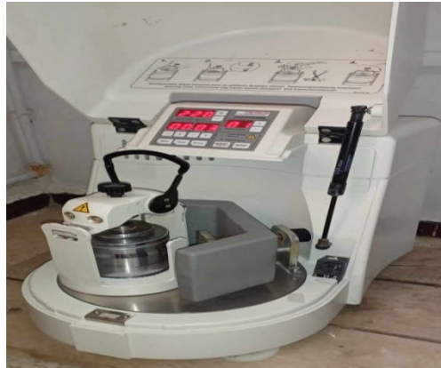
Figure III.7 : machine de broyage.
