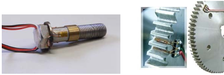
Figure.IV.42. Control of deformations in a clamping screw and a polish under full load.
