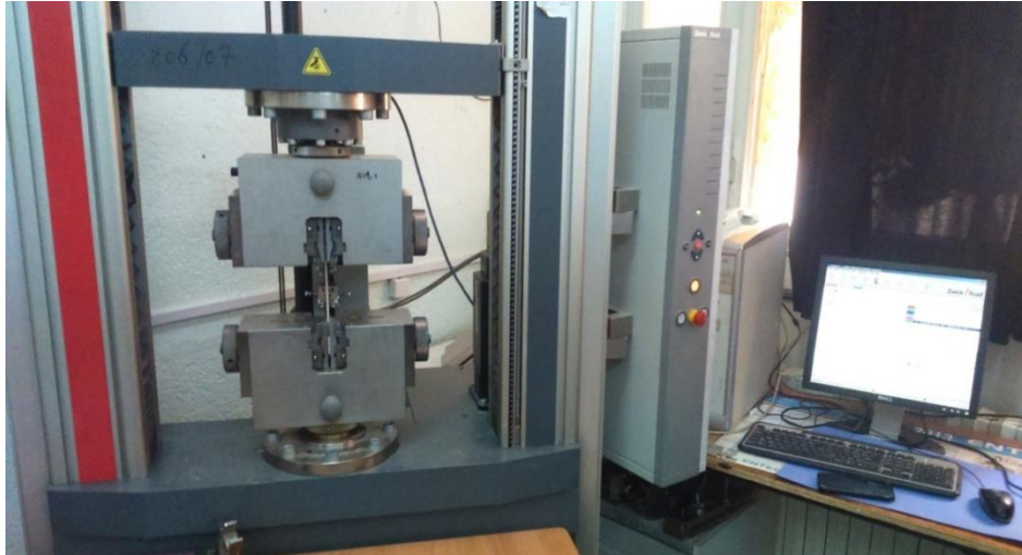
Figure IV. 16. Machine de traction /compression Zwick- Roell De type z100.
