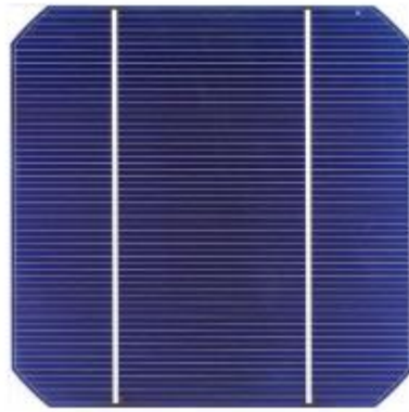
Figure II.3. Cellule en silicium monocristallin.
