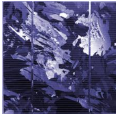
Figure II.4. Cellule en silicium Polycristallin.
