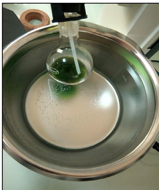
Figure 38. Extraction operation by rotary evaporator.
