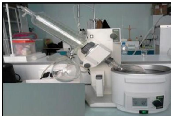
Figure 31. Rotary evaporator (BÜCHI R - 210).
