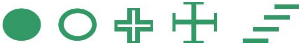
Figure 2.6 .— Examples of Frequency Selective Surfaces (FSS).
