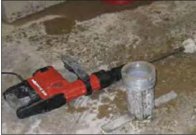
Figure I. 15 : Marteau vibrant (Harrington 2010).
