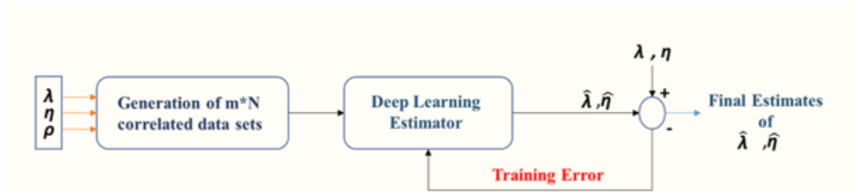
FIGURE 5.1: Synoptic diagram of the deep learning-based estimator for correlated Pareto type II clutter.
