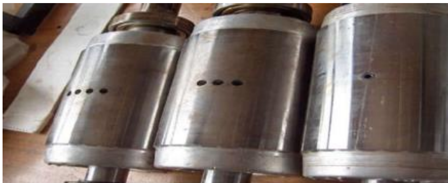
Figure 6 Ruptures de barres [10].
