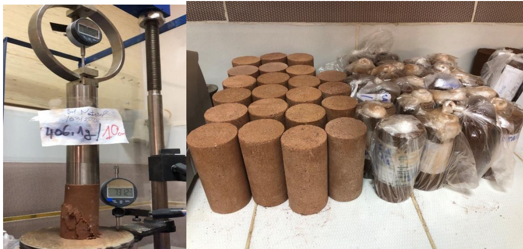
Figure II.11 : Essais de compression simple
