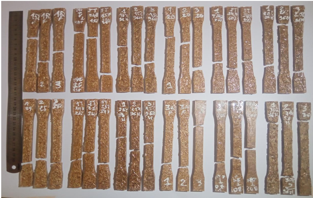
Figure III.7: Samples after tensile test
